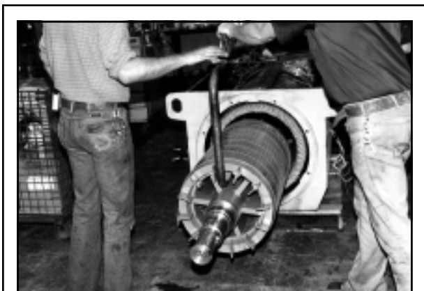
Figure 17. Rotor removal using a rotor removal tool.
