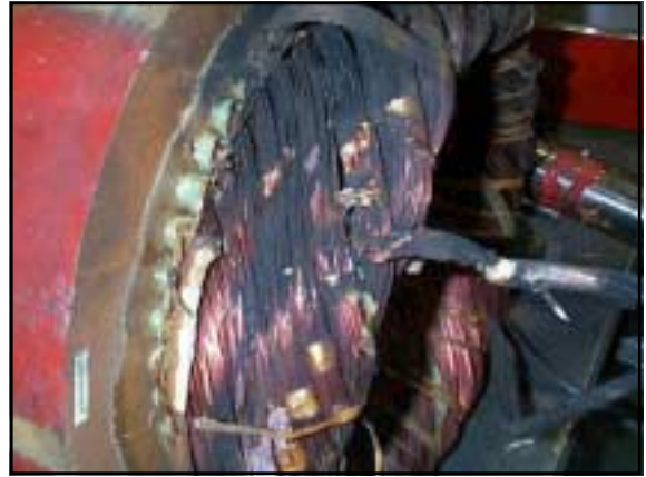
Figure 34. "Buried coils" in a lap winding.
