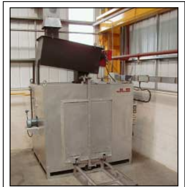
Figure 23. Controlled temperature burnout oven.
